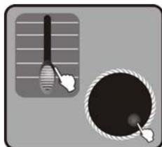
4. Move **FADERS1-24** and use Jog wheel **#3**, **#4** to change the center position of PAN, TILT where you desired. (The codes of the channel feature of ARRT CODE are "P", "PF", "T", "TF" in the fixtures bank) for the convenience to check other channels, there would be some output of the channels, but the channel output will not be stored in the center.
