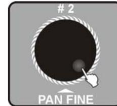
3. Use Jog wheel **#2** to chose the channel of MIDI (0-16) , it's enlarge mode when the value of the MIDI channel is 0, so MIDI can receive the information of 1-16 channels.
