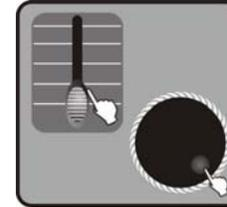
3. Slide **Faders 1-24** or use the **CENTER** or **PRESET** or **SCENE** have saved to change the output of each channel. You can also use the jog wheel #1, #2 to control the PAN, PAN FINE or use the jog wheel #3, #4 to control TILT, TILT FINE.
