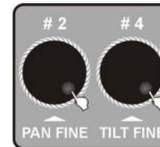
4. Turn Jog wheel **#2** to change the position of the cursor, and Jog wheel **#4** used to reverse the channel.
