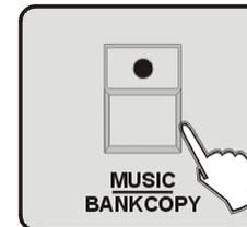
6. Press the button **MUSIC/BANK COPY**, all LEDs and the Segment Display will blink for three times briefly indicating this operation, then the LCD will show the number of the being copied bank and the bank is being copied to and the scene number of the programmed scene.
