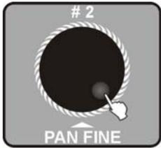
4. Use the Jog wheel #2 to select the position of inserted steps.
