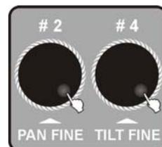
5. After 3 seconds, use jog wheel **#2** to select the fixtures of the first group, and jog wheel **#4** to select the fixtures of the second group. When you turn the jog wheel **#2** or **#4**, the cursor will switch between the first and second group. The fixtures of this two group will be selected in turn, and the unit will act differently when it be selected.
