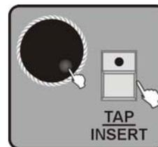
4. Use Jog wheel **#3** or **#4** to adjust current **FADE TIME** or **WAIT TIME**, or use **TAP/INSERT** Button to adjust the speed of the scene.
